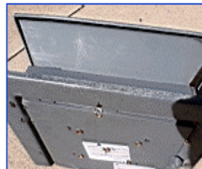
Post Test Impact Bottom Side
